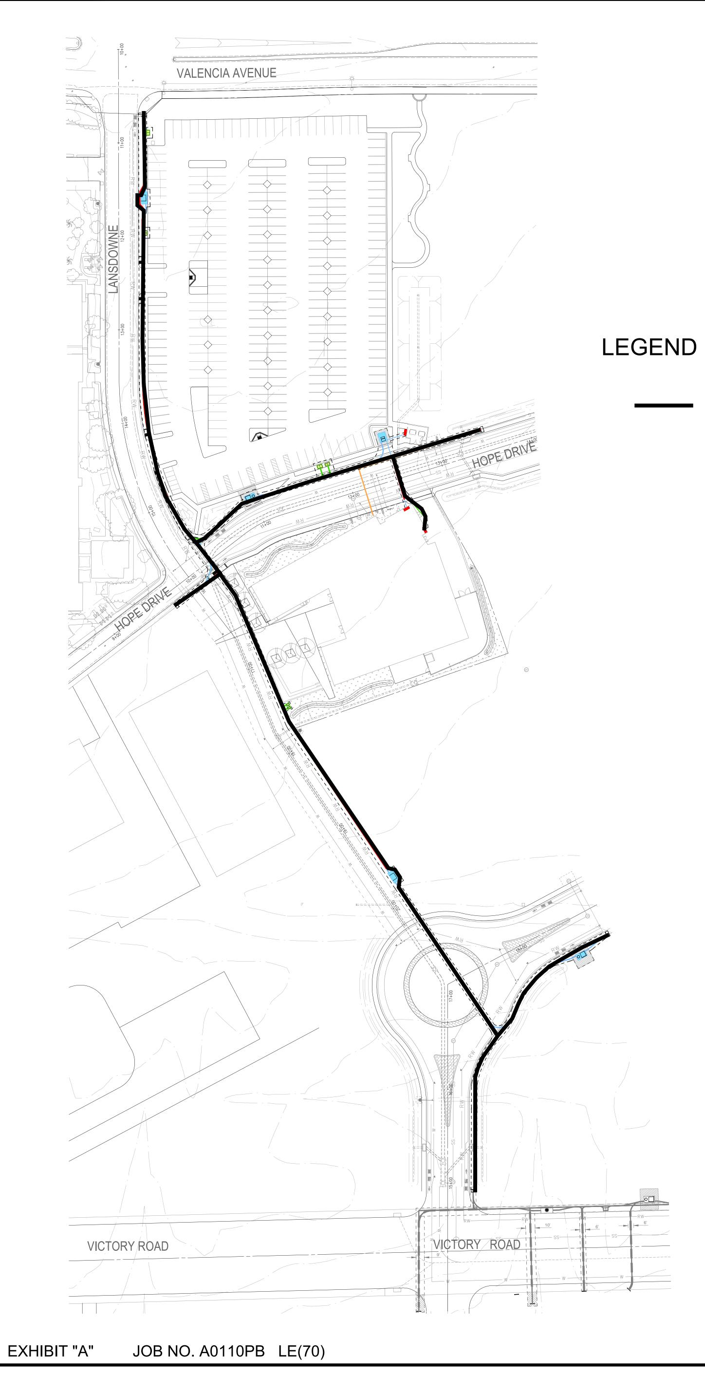
CENTERLINE OF A 6' EASEMENT TO PACIFIC BELL TELEPHONE COMPANY DBA AT&T CALIFORNIA
